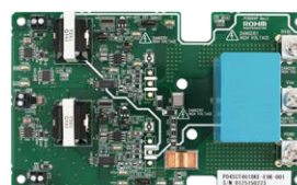
Solution board for easy evaluation of SiC power devices
