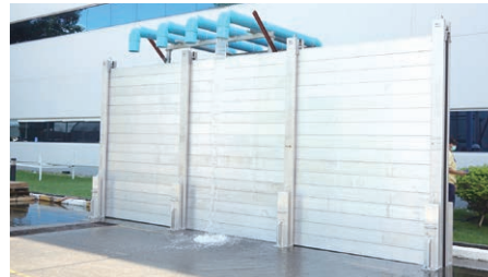
Flood wall assembly training at the manufac- turing site in Thailand
