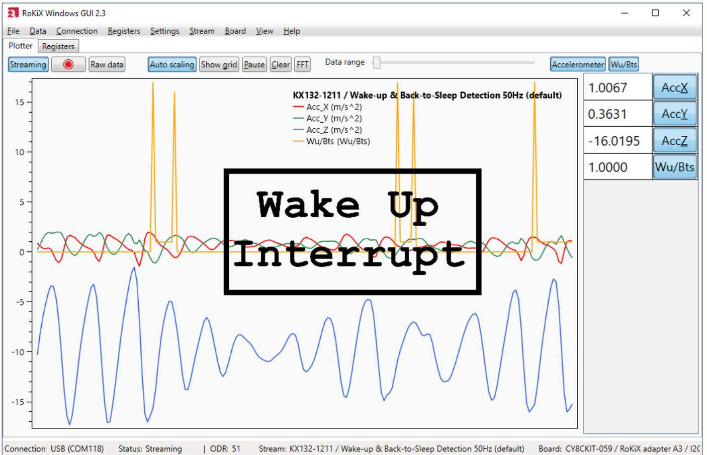
Figure 65. The plotter view with wake up triggered.
