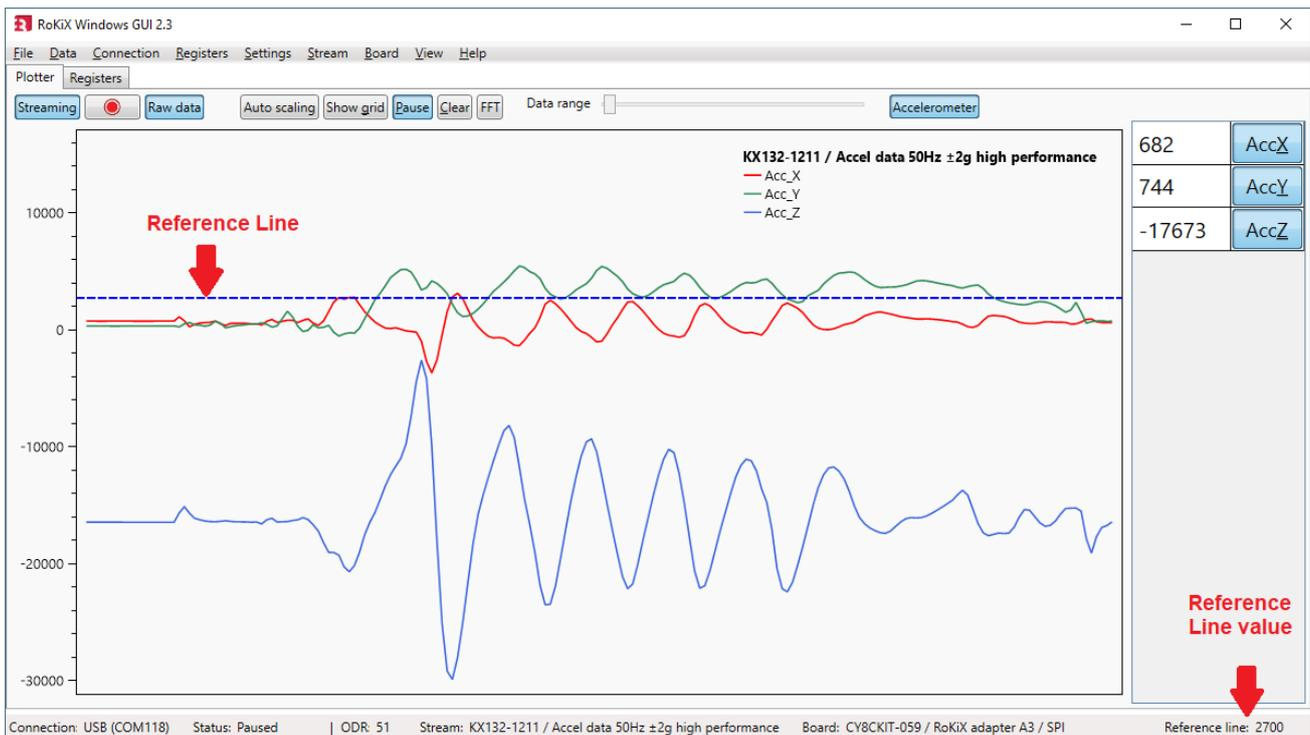
Figure 35. Plotter view with reference line enabled.
