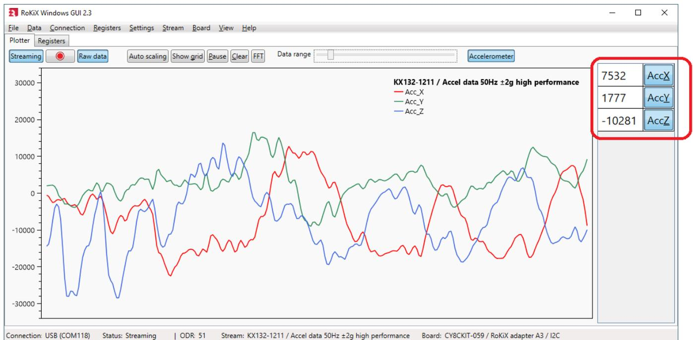
Figure 32. Plotter view with Sub Channel View and Digital Output Enabled
