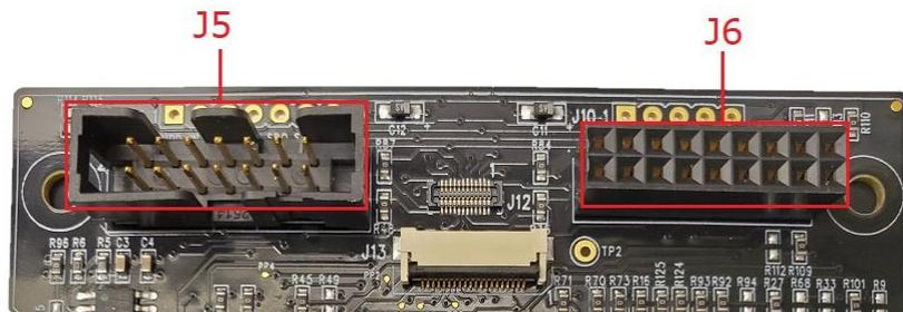
Figure 9. RoKiX Digital Evaluation Board Interface Headers
