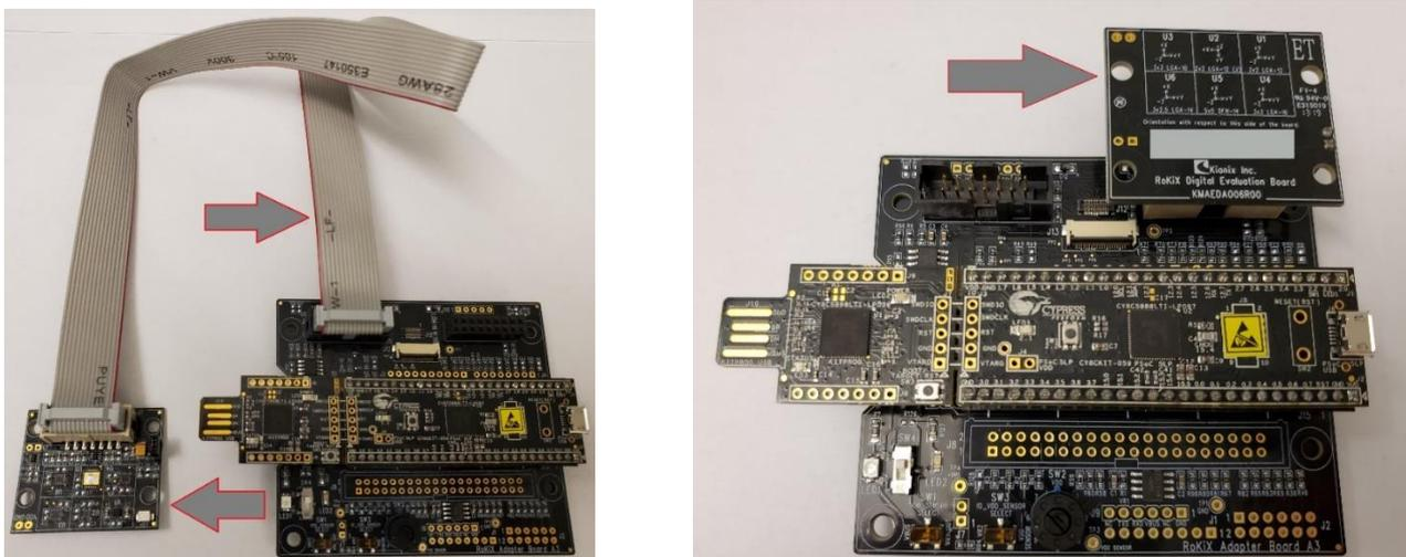
Figure 10. Interface with RoKiX Digital Evaluation Board
