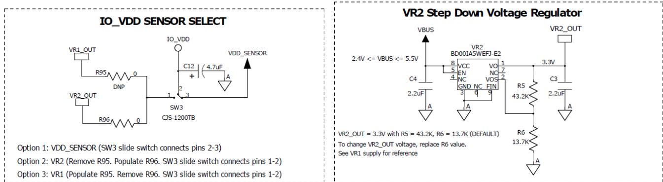
Figure 5. IO\_VDD Sensor Select and VR2 Voltage Regulator
