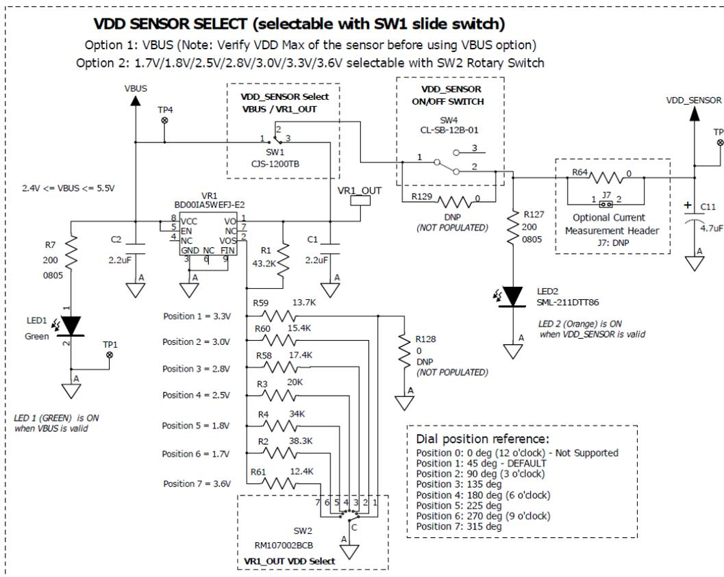
Figure 4. *RoKiX Adapter Board A3* VDD Sensor Select
