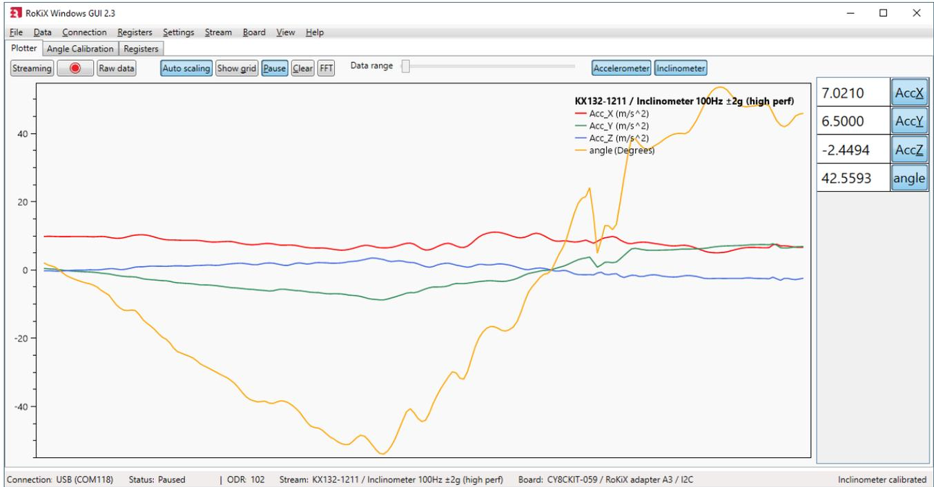
Figure 50. Plotter view with KX132-1211 inclinometer stream.
