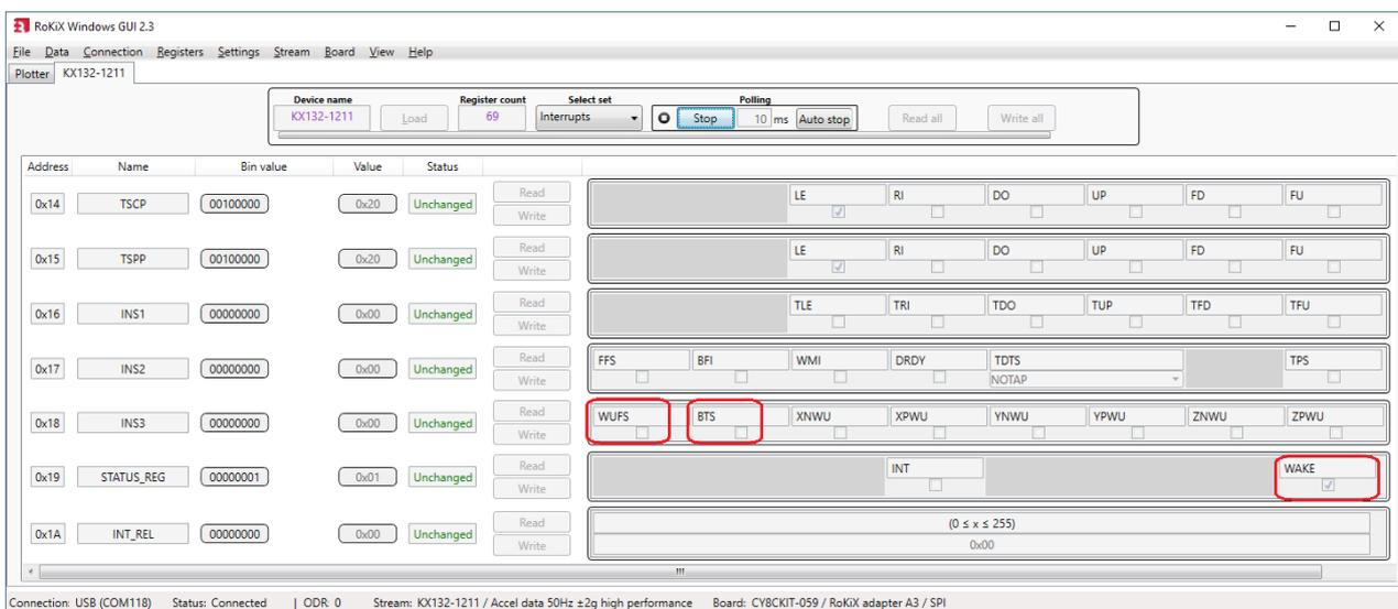
Figure 62. Wake-Up / Back-to-Sleep Interrupt Detection Register Set
